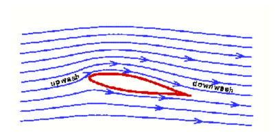
Fig 4 True airflow over a wing with lift, showing upwash and downwash.
