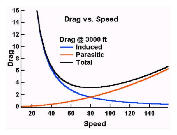
Fig 12 Drag versus speed.
