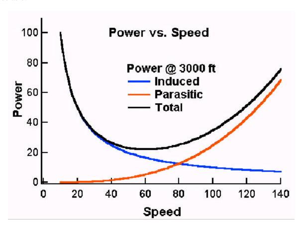
Fig 11 Power requirements versus speed.
